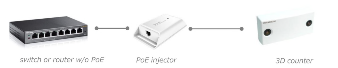
Figure 7: Connecting to Network Equipment that does not have PoE capability:
