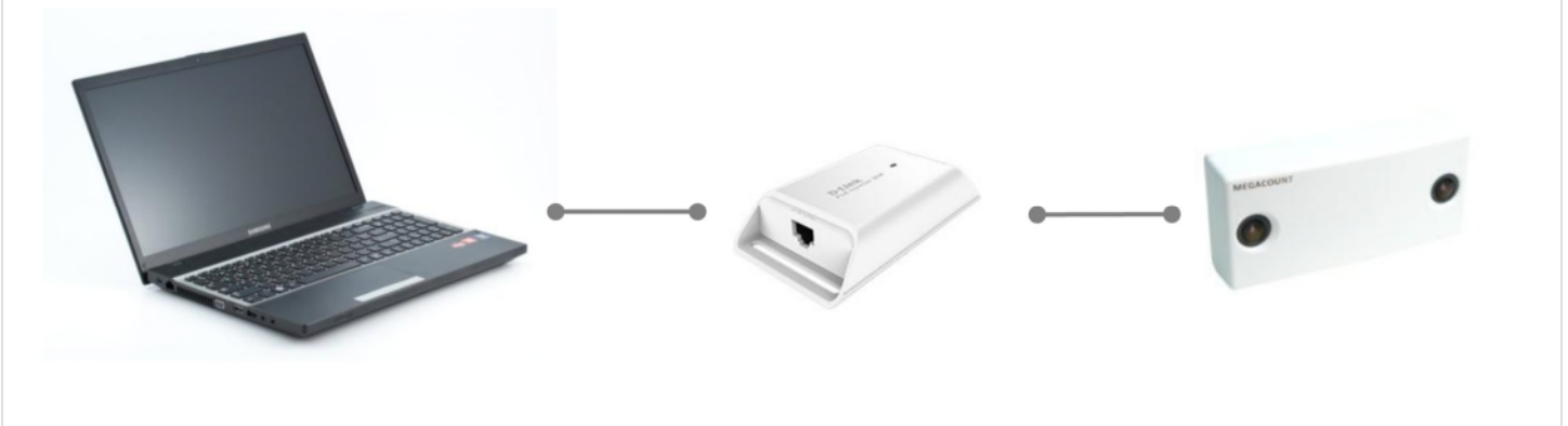
Figure 11: Connecting the People Counter Directly to a PC:
